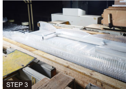
STEP 3 Clamp the package U-shaped wooden guard strips to the countertop with the countertop packaging machine
