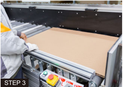
Place honeycomb-paper cardboard at the bottom
