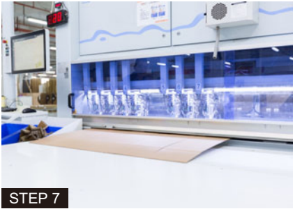
Cut the cartons into suitable size
