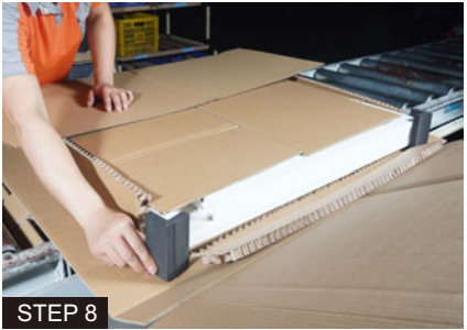
Fill with honeycomb-paper cardboards, protect the four corners with EVA foam
