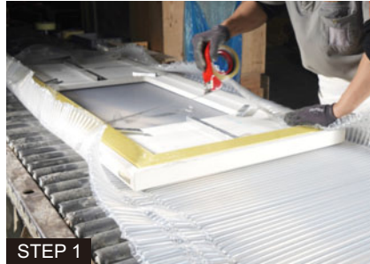
STEP 1 Wrap the countertop with an air column bag for shock absorption
