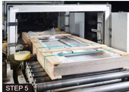
STEP 5 Tighten the countertop with plastic belts
